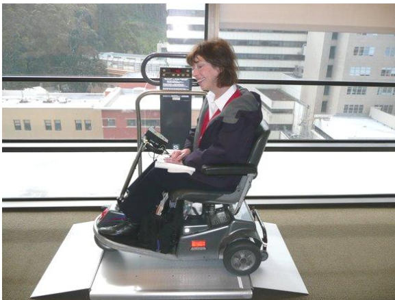
Figure 4. x. Above is a sample picture of a Scaletronix Oversized Wheelchair Scale, 6702W with a scooter user. This wheelchair scale is large enough to accommodate a scooter user. For more information on wheelchair scale platform sizes, refer to page 19, Resources .
